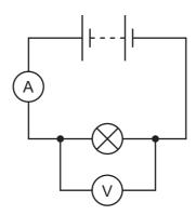
The ammeter reading is 2.0 A and the voltmeter reading is 6.0 V.
